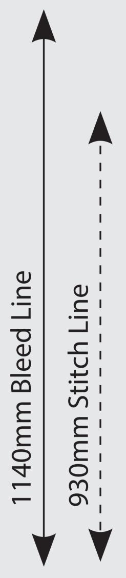
Note: 'Halfwalls' are folded over a crossbar and stitched onto the inside. For front printing, the artwork should be up to the designated 'top of the halfwall line'. Inside wall artwork should finish at the stitching line.
